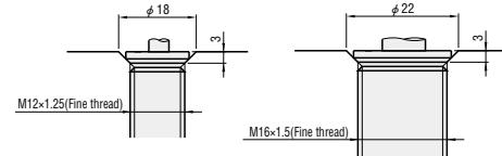
Machine the mounting screws in the manner listed above and ensure the MGSM's flange and the mounting surface are in contact.
