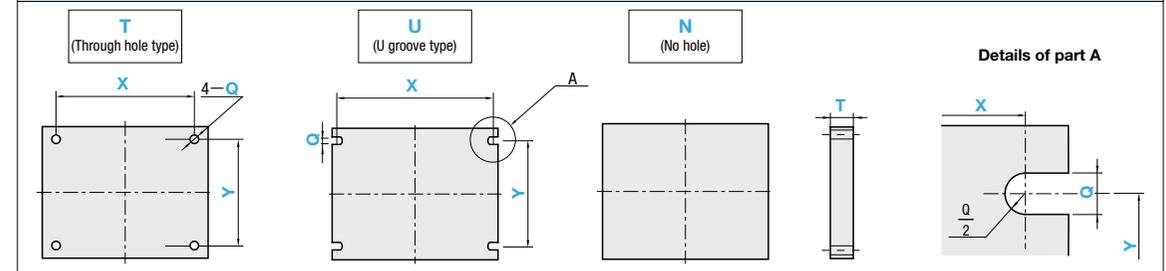
※To ensure strength, hole cannot be set on 4mm or less departing from each edge.
